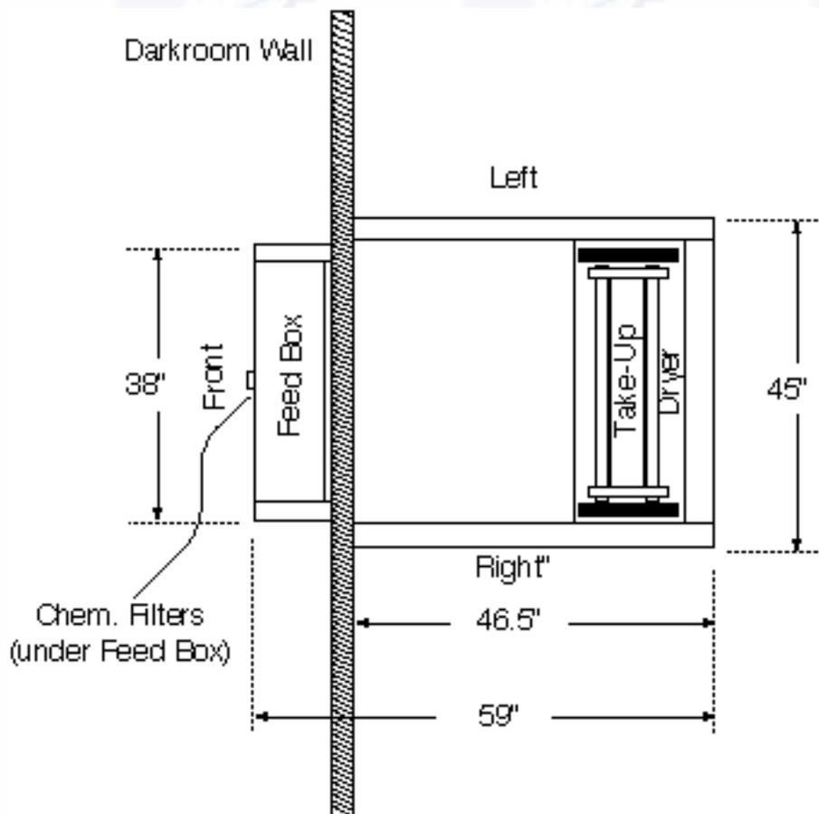
Cut sheet material exits on top of processor.
