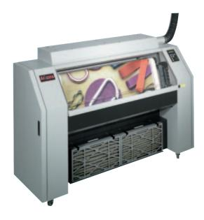
**Printing Method** Drop-on-demand piezoelectric inkjet with 384 nozzles (3 × 128 print heads) per color
