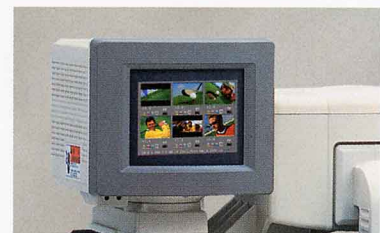
The digital monitor displays positive images of the negatives as well as error messages and instructions.
