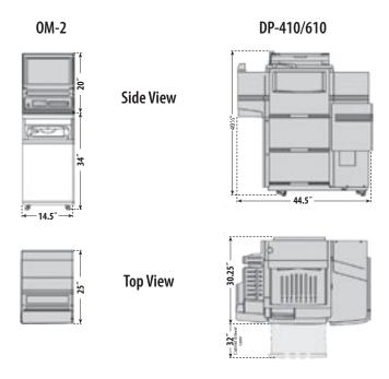
The Complete dDP 421/621 system consists of an OM-2 and a dDP-410/610.
