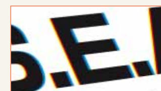
Conventional print Colors of R, G and B appear by blur at the edge of black letters in white background.
