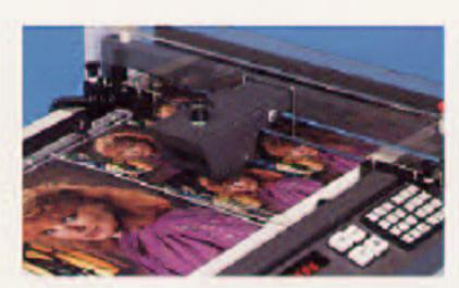
Pickups and pressure roller are easily adjustable. Adjustable pickup lets you center cut marks between double cut.
