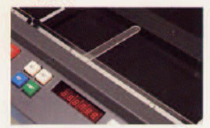
Optional Fine Point Control allows operator to compensate for inaccurately spaced prints on unmarked rolls.
