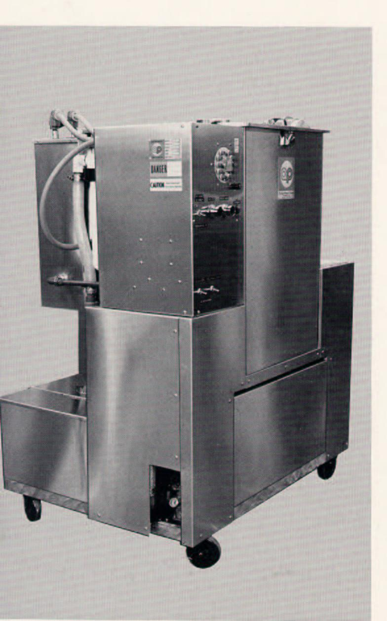
The R-2 Rack Washer has a distinct advantage over ultrasonic types of cleaners which vibrate mechanical parts loose and therefore require careful checking and retightening after the cleaning process is complete. There are also obvious thoroughness and labor-saving benefits over hand washing and scrubbing.
